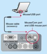
•Use a USB mouse cable to connect the projector to the USB port of a computer.
