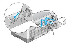
6. Gently insert the end of the paper into the printers as far as it will go, flush with the right edge guide. Slide the left edge guide against the left edge of the printer.
