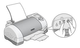
4. Release only the <sup>(b)</sup> power button. After the nozzle check starts, then release the <sup>(b)</sup> maintenance button.
