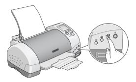
The printer will start cleaning the print head and the process light will begin flashing. Print head cleaning takes about thirty seconds to complete.
