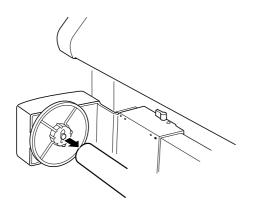
4. Turn the lock lever to the front to lock the movable unit.
