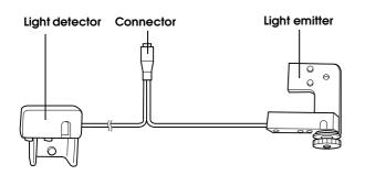
1. Set the sensor unit's light emitter in the bottom of the drive unit, and then secure it with a screw.
