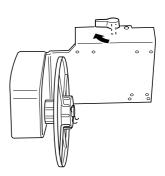
2. While holding the movable unit, attach the movable unit stopper on the bottom of the movable unit. Snap the two protrusions of the stopper into the movable unit, so the stopper does not fall off.
