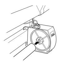
3. Insert the flanged knob on the movable unit into the other end of the take-up reel core.
