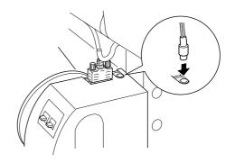
4. Fasten the cable using the cable clamps provided. Use as many of the clamps as necessary to secure the cable. You may need to do this from the back of the printer.
