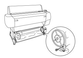
2. Set the sensor unit's light detector in the base unit's bottom left side, and then secure it with a screw.
