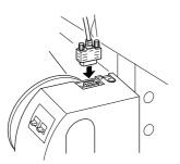
4. Plug the other end of the cable connector into the connector on the back of the printer as shown below, then tighten the screws on both sides of the connector.
