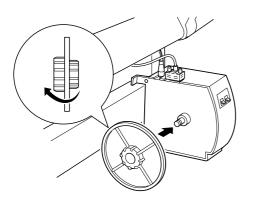
5. Replace the cap and fastener, which you removed in step 2, on the drive unit.
