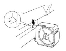
2. Tighten the two screws to attach the drive unit to the printer securely.
