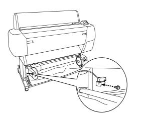
3. Plug the connector of the sensor unit cable into the socket located at the top rear of the control box on the drive unit.
