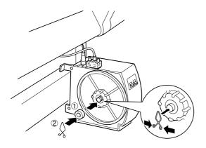
6. Remove the fastener from the movable unit. Next, remove the flange.
