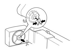
9. Install the 2-inch take-up reel core in the auto take-up reel unit in the same manner as described in "Installing the 3-inch take-up reel core" on page 5.
