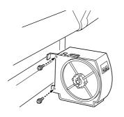
3. Plug the cable connector into the connector on top of the control box of the drive unit, then tighten the screws on both sides of the connector.
