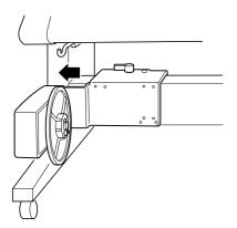
2. Slip one end of the take-up reel core over the flanged knob on the drive unit.
