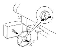
7. Reverse the flange so that the smaller knob is positioned on the outside, then replace it on the movable unit.
