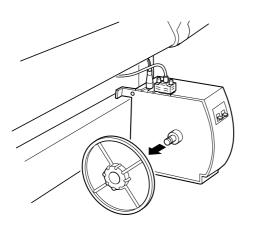
4. Reverse the flange so that the smaller knob is positioned on the outside, then replace it on the drive unit.
