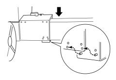
3. Tighten the two screws to attach the movable unit to the horizontal strut.
