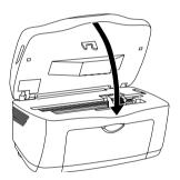
The print head moves and ink charging begins. The On light flashes while ink charging is in progress. When the On light stops flashing, ink charging is completed.
