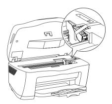
3. Open the document cover and slide the carriage lock lever, as shown in the illustration below, to lock the scanner carriage.
