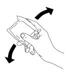
5. Pinch the sides of the ink cartridge that you want to replace. Lift the cartridge out of this product and dispose of it properly. Do not take the used cartridge apart or try to refill it.
