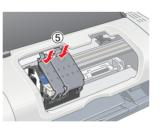
Install all ink cartridges. The printer will not work unless all cartridges are installed properly
