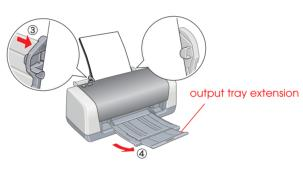
To adjust the left edge guide, hold down the locking tab and slide the guide against the paper stack.
