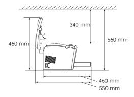
☐ If you install the optional lower paper cassette, you will need an additional 130 mm (5.1 inches) in height. If you install the optional Face up tray, you will need an additional 200 mm (7.9 inches) in back of the printer.
