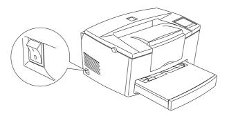
2. Insert the power cord into the back of the printer. Then plug the other end into a properly grounded electrical outlet.
