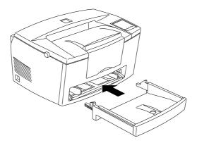
2. Fan a stack of paper (up to 150 sheets), then align the edges by tapping the stack on a flat surface. With the paper's printable side facing up, place the stack into the tray and push it all the way in. Slide the paper guide against the right side of the paper stack.
