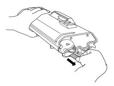
4. Insert the pins on each side of the cartridge into the grooves inside the printer, and slide the cartridge gently into place. Then push down the handle until the cartridge is horizontal.
