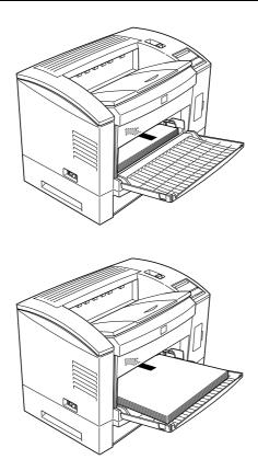
3. Adjust the paper guides to match the size of your paper. Load the stack of paper into the MP Tray with the printable side up.
