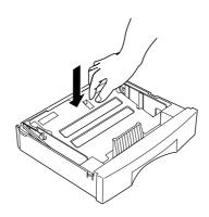
3. Fan a stack of paper and tap it on a flat surface to even the edges. Insert the paper face-up into the tray with the corners of the paper underneath the tabs.
