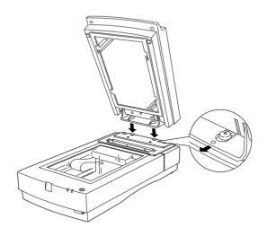
4. Insert the two installation screws provided with the Transparency Unit into the holes as shown below, and then tighten the screws with a coin.
