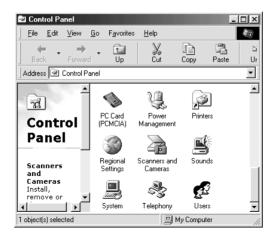
2. Select a scanner you want to use from the installed scanners and cameras list in the Scanners and Cameras Properties dialog box. Click Property, and then click the Utility tab.
