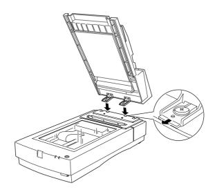
4. Insert the installation screws included with your Automatic Document Feeder into the holes in the scanner, then use a coin to tighten them.
