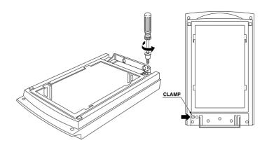
3. Screw the shipping screw into the storage hole as shown.
