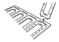
2. Insert a strip of film in the film strip holder, making sure the glossy (smooth) side of the film is facing down.
