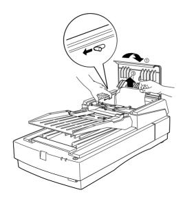
After removing the jammed paper, close the document feeder cover and make sure the READY light is on and not flashing, and the ERROR light is off.
