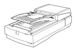
2. Insert the paper stack into the Automatic Document Feeder until it meets resistance. Make sure that the side you want to scan is facing up.
