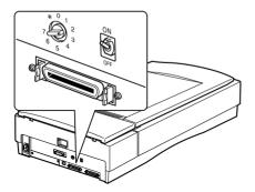
The SCSI ID rotary switch is located at the rear of the scanner.
