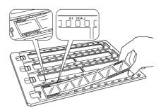
3. Replace the strip cover that you removed in step 1. Repeat steps 1 through 3 for all the film strips you scan.
