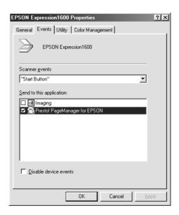
2. You can see the Start Button is listed as the scanner event. Make sure the check box of the application you want to assign to the ⊈ Start button is selected and all other application check boxes are clear in the Send to this application list.
