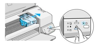
The printer starts cleaning the print head and the  $\circ$  power light begins flashing. Print head cleaning takes about one minute to complete.
