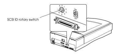
If you add the scanner to a system in which one of your SCSI devices already has a SCSI ID of 2, change the ID number to an unused number using the rotary switch. See the table below as a guide.
