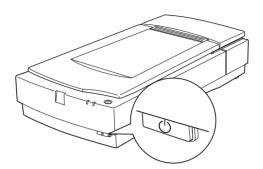
2. If the power cord is not attached to the scanner, connect it to the AC inlet on the back of the scanner, and plug the other end into a properly grounded electrical outlet.
