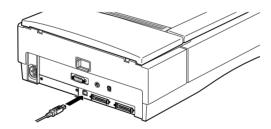
2. Connect the other end of the cable shown below to the USB port on your computer, or USB hub.
