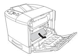
If the optional Duplex Unit is installed, lift up the Duplex Unit. Hold it and gently pull out any sheets of paper. Be careful not to tear the jammed paper.
