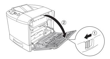
5. If the optional Duplex Unit is not installed, gently pull out any sheets of paper. Be careful not to tear the jammed paper.
