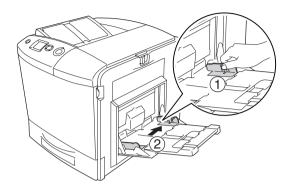
4. Load a stack of the desired paper on the center of the tray. Make sure to load it with the printable surface down.
