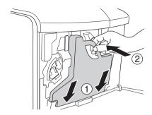
5. Remove the filter from the printer.
