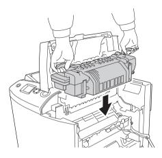
11. Turn the handles on both sides of the fuser unit to lock them.
