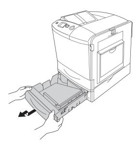
10. Gently pull out any sheets of paper that have fed part way into the printer.
