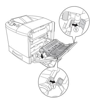
8. Pull the upper part of the Duplex Unit upward and secure the Duplex Unit to the printer with the two provided screws.
