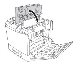
6. Hold the guide up by holding the green tab, and gently pull out any sheets of paper. Be careful not to tear the jammed paper.
