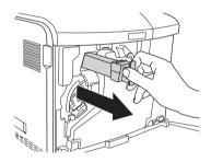
6. Take the new filter out of its package. Insert the new filter to the printer.
