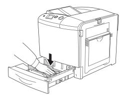
3. Load a stack of paper into the paper cassette. Make sure to load it with the printable surface up.
