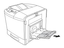
**Note:** When you use A4, Letter or larger sizes of paper, unfold the expansion tray 2 by lifting it up.
