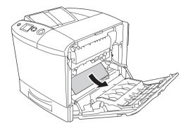
If the optional Duplex Unit is installed, lift up the Duplex Unit. Hold it and gently pull out any sheets of paper. Be careful not to tear the jammed paper.
