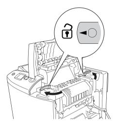
5. Lift the fuser unit out of the printer as shown below.
