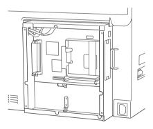
5. Secure the Hard Disk Drive with the four screws provided.
