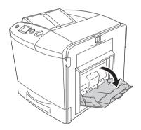
3. Push the latch on cover A to the left and open the cover.
