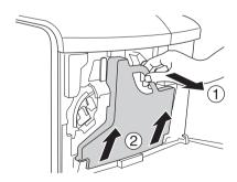
5. Take the cap off and cover the hole for the waste toner collector with it.
