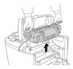
6. Take the new fuser unit out of its package and remove the protective cover.
