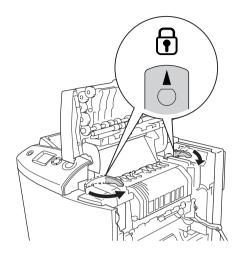
**Note:** Make sure that the locks are completely in the locked position.
