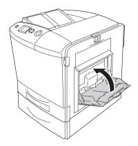
*Note:* Close the expansion trays, if needed, before closing the MP tray.
