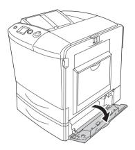
5. Fasten the optional paper cassette unit to the printer with the provided plates and screws.
