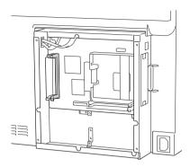
5. Insert the memory module vertically into the slot until the clip comes out. Make sure that the left slot has a module at all times.
