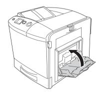
*Note:* Close the expansion trays, if needed, before closing the MP tray.
