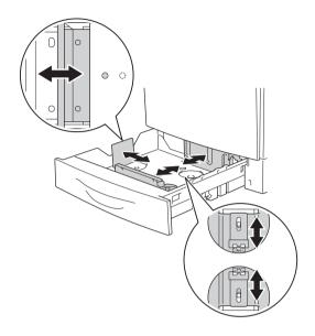
5. Secure the three paper guides with the three screws.
