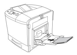
Gently pull out any sheets of paper that have fed part way into the printer.
