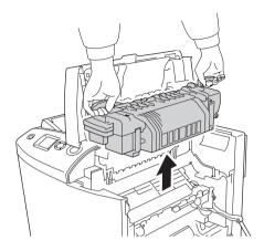
9. Remove the paper. If the paper is still jammed in the fuser, turn the green knob on the back of the fuser to remove it.
