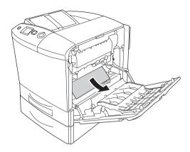
If the optional Duplex Unit is installed, lift up the Duplex Unit. Hold it and gently pull out any sheets of paper. Be careful not to tear the jammed paper.
