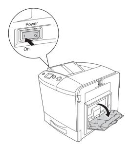
2. Pull out the expansion tray on the MP tray to accommodate the size of the paper you want to load.
