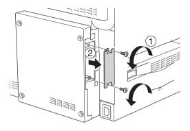
3. Slide and push the interface card into the slot firmly, then fasten the screw as shown below.
