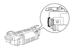
10. Lower the fuser unit into the printer making sure that the guide posts slide into the holes on the bottom of the unit.
