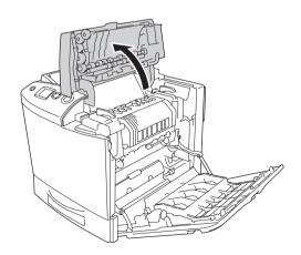
4. Turn the handles on both side of the fuser unit to unlock them.
