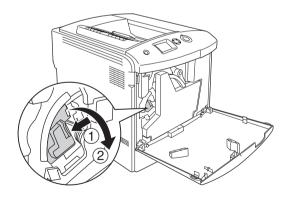
4. Remove the empty toner cartridge from the printer.
