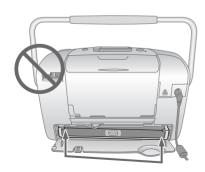
9. Set the lever to the Lock position by sliding it in the direction shown.
