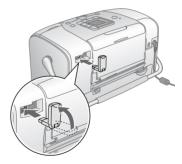
2. The Adapter's light comes on for one second. If the LED does not turn on, disconnect the Adapter from the printer, then reconnect it.
