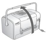
5. Open the cartridge compartment cover on the back of PictureMate.
