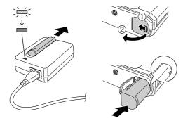
The battery is fully charged when the red light on the charger turns off.
