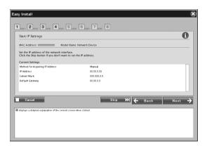
14. Select Auto or Manual to assign the IP address to the network interface.
