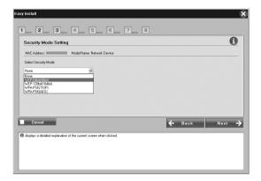
When you select WEP-64 bit (40 bit) or WEP-128 bit (104 bit), the WEP Key Settings screen appears.
