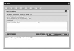
13. Select Auto or Manual to assign the IP address to the network interface.
