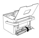
3. Set the cartridge lever in the Release position by pulling it to the left. The photo cartridge will be ejected about halfway out of the cartridge holder.
