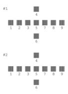
Look at the alignment pattern in each set and find the patch which is most evenly printed, with no noticeable streaks or lines. 10. Press the ▲ or ▼ button to highlight the number for the best pattern (1 to 9) for set #1, then press the right soft key.
