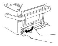
Pull the cartridge out of PictureMate and dispose of it properly.
