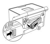
3. Attach the battery cover as shown below.
