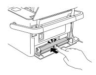
7. Set the lever to the Lock position by sliding it to the right.
