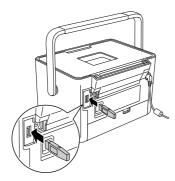
2. The Adapter's light comes on for one second. If the LED does not turn on, disconnect the Adapter from PictureMate, then reconnect it.
