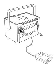
☐ For a flash memory drive, plug it into the EXT. I/F port on the back of PictureMate.
