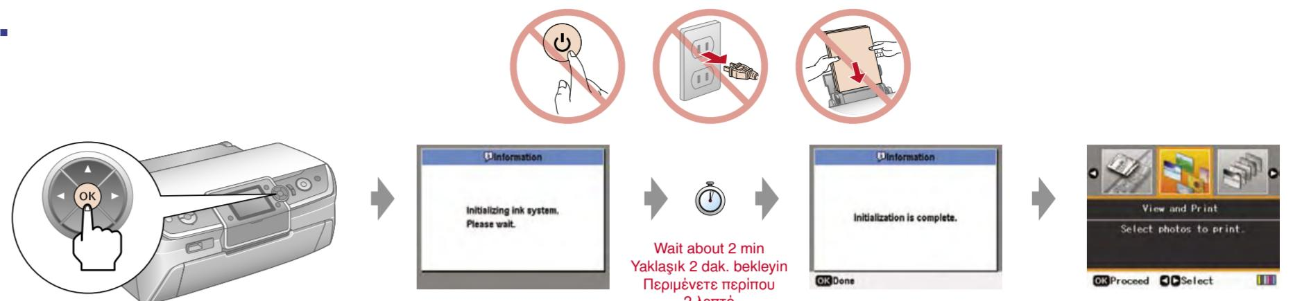
**Note:** The ink cartridges first installed in your printer will be partly used to charge the print head. Subsequent ink cartridges will last for their full rated life.
