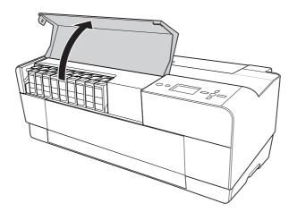
4. Press the ink eject button, then the ink cartridge is slightly pushed out.
