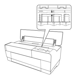
4. If the problem still occurs, clean it using a soft, clean cloth dampened with mild detergent. Then, wipe the inside of the printer dry with a dry, soft cloth.
