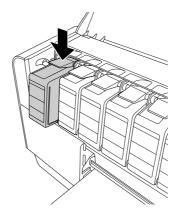
5. Carefully pull the expended cartridge straight out of the slot, and dispose of it properly.
