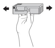
8. Hold the ink cartridge with the arrow mark facing up and pointing to the rear of the printer, and then insert it into the slot as far as it will go until it clicks.
