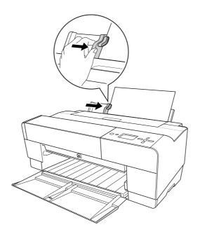
6. Guide the paper into the slot and feed it into the printer until it meets resistance. Maintain a constant pressure against the paper (approx. 3 seconds) until you feel the printer pull the paper in slightly.
