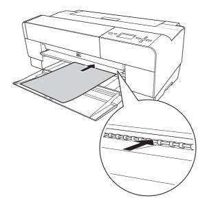
4. Adjust the right edge of the paper resting against the right side of the front manual tray, and also align the bottom edge of the paper with the white line.
