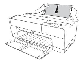
The printer automatically feeds the paper to the printing position.
