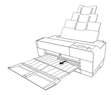
If necessary, open the top cover, and remove the jammed paper.
