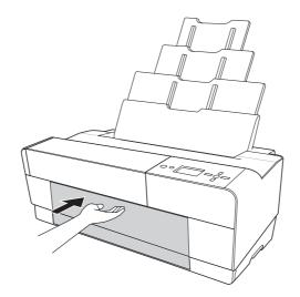
4. Raise and pull out the output tray extension while pulling it out.
