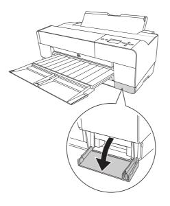
3. Put your hand on the handle of the maintenance cartridge, then push up the maintenance cartridge and gently pull it outward.
