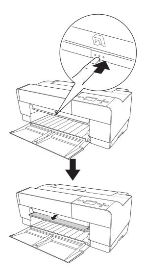
3. Insert a sheet to where paper is usually ejected.
