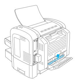
3. Close the Duplex Unit's lower cover. The jammed page's print data is automatically reprinted.
