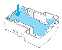
4. Tap the edges of the paper stack on a flat surface to even the edges, and then set it back into the paper tray.
