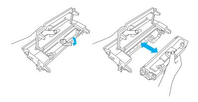
5. Remove the new developer cartridge from its bag. While holding the cartridge horizontally, gently shake it a few times from side to side and then from front to back to distribute the toner evenly.
