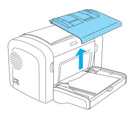
3. Gently pull out any sheets that have fed part way into the printer.
