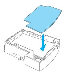
6. Insert the loaded paper tray back into the unit.
