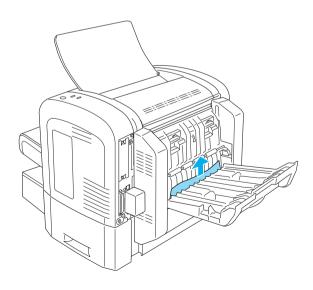
3. Close the Duplex Unit's upper cover. The jammed page's print data is automatically reprinted.
