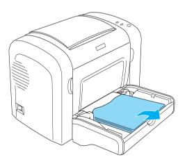
3. Gently pull out any sheets that have fed part way into the printer.
