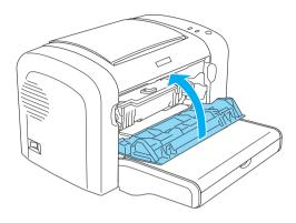
Whenever you replace the developer cartridge, you should also clean the paper roller as described in "Cleaning the paper path rollers" on page 338.
