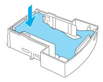
4. Fan a stack of paper and tap it on a flat surface to even the edges. Then load it into the paper tray.
