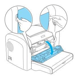
3. Remove the developer cartridge.
