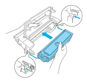
7. Hold the photoconductor unit's casing by its handle and insert it into the printer. Slide it gently into the opening until it locks into place.
