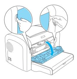
3. Remove the developer cartridge and the photoconductor unit by holding the photoconductor unit's casing by the handle and pulling it out of the printer.
