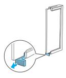
7. Replace the printer's right side cover as shown below.
