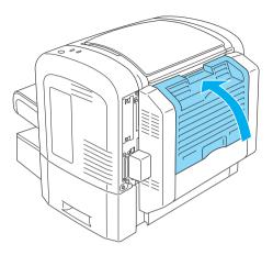
10. Connect the cable to the Duplex Unit connector on the printer, and then close the rectangular covering.
