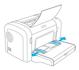
2. Insert a single sheet of paper, with the printable side up, as far as it will go into the manual feed slot above the tray cover. Adjust the paper guides to match the paper size you are using.
