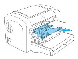
4. Turn the release lever in the clockwise direction to release the developer cartridge, and then pull it out from the photoconductor unit's casing.
