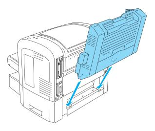
7. Carefully push the unit against the printer, making sure that the hook on the top-right corner is firmly inserted into the hole on the printer.
