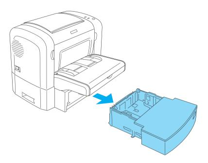
2. Remove any folded or jammed paper from the paper tray and from the inside of the cassette unit, and discard any curled or wrinkled sheets.
