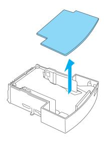
3. Press down on the plate in the paper tray until it locks into position.
