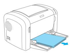
2. Gently pull out any sheets that have fed part way into the printer.
