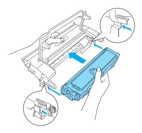
8. Hold the photoconductor unit's casing by its handle and insert it into the printer. Slide it gently into the opening until it locks into place.
