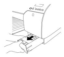
4. Put the used maintenance tank in the plastic bag provided.
