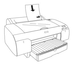
The printer automatically feeds the paper to the printing position.
