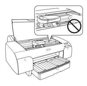
7. Slowly take your finger off the side pin, and carefully remove the old cutter from the printer.
