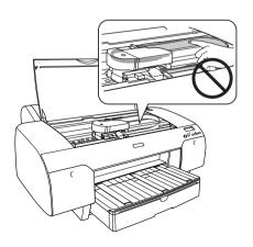
3. If the back of a printout is soiled, carefully clean the platen (the gray part) using a soft, clean cloth.
