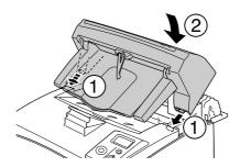
4. Secure the screws at both ends of the bottom of the Stacker.
