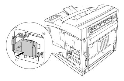
8. Secure the drive using the screws that come with the drive.
