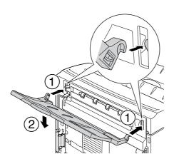
2. Push up the paper path lever and pull out the extension tray.
