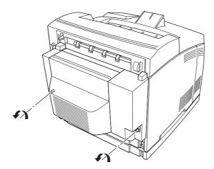
3. Press the unlock button to unlock the hooks, then remove the unit from the printer.
