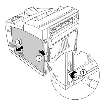
3. Loosen the two screws using a screwdriver. Then hold the tab on the top of the shield cover and remove the cover.
