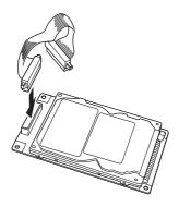
6. Connect the other end of the cable to the Hard Disk Drive socket on the circuit board.
