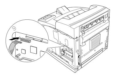
7. Insert the bottom side of the Hard Disk Drive into the printer and push it to set it in the correct position.
