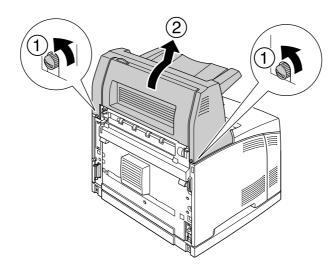
4. Insert the right and left tabs of the top cover into the holes on the top of the printer, and then tighten the two screws.
