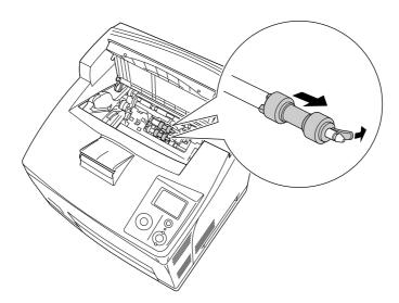
4. With a clean damp cloth, wipe the pickup roller's rubber parts.
