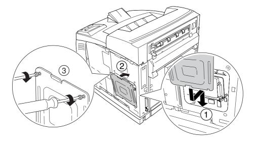
10. Reattach the right side cover to the printer as shown below. Then, tighten the screw on the back of the printer.
