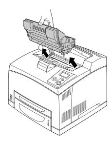
3. Take the new imaging cartridge out of its package and gently shake the imaging cartridge as shown below.
