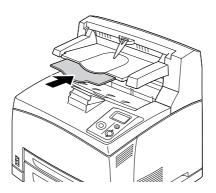
3. Loosen the screws on both sides of the Stacker, and while holding up the Stacker, remove the right and left tabs from the holes on the top of the printer.
