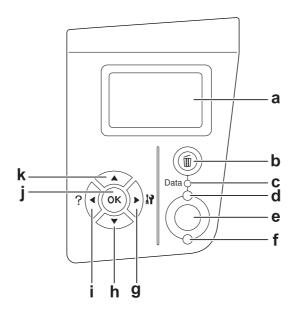
a. LCD panel Displays printer status messages and control panel menu settings.
