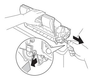
5. Insert the new imaging cartridge all the way until it stops.
