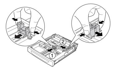
4. Load a stack of the desired paper on the center of the cassette with the printable surface facing up. Then slide the side paper guide while pinching the knob until it is against the right side of the stack to get a snug fit.
