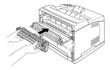
8. Lift up the two levers at either side of the fuser unit to lock it.
