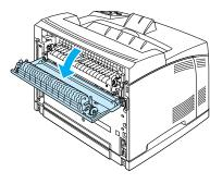
When the optional Duplex Unit is installed, open the Duplex Unit's cover before opening cover B.
