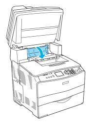
7. Lower the scanner unit to the original position.
