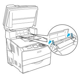
4. Hold the guide up by holding the green tab, and gently pull out any sheets of paper. Be careful not to tear the jammed paper.
