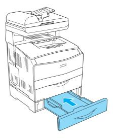
If the jammed paper is not visible inside the optional paper cassette or to check if there is any jammed paper inside cover G, proceed to step 4.
