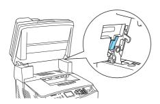
2. Open cover C, then raise the two green levers on the fuser unit to unlock it.
