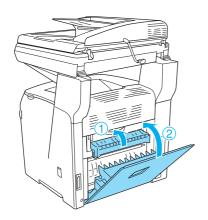
6. Push down the two green levers on the fuser unit, then close cover C.
