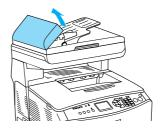
2. Gently pull out any sheets of paper with both hands. Be careful not to tear the jammed paper. If you cannot pull out the jammed paper, proceed to the next step.
