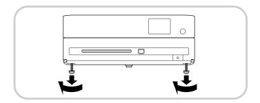
If you extend the foot and tilt the unit, the image will have keystone distortion. Reshape the keystone distortion as follows:
