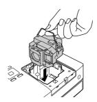
Tighten the lamp attachment screws firmly.
