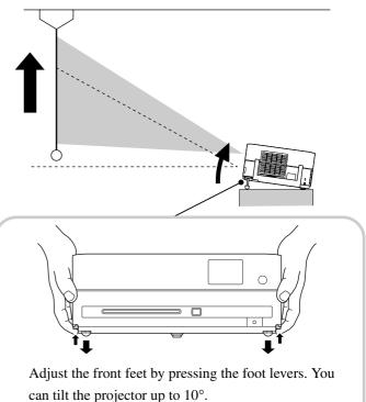
Adjust the feet in such a way that the unit is level.
