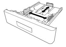
When the size of the paper that is loaded is bigger than A4, detach the green stopper and attach it to the paper guide.
