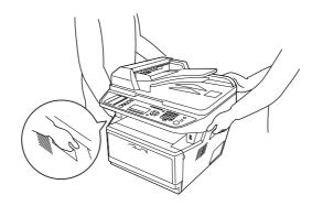
4. Align the corners of the printer and the unit, then lower the printer gently onto the unit so that the connector and two pins on the top of the unit fit into the terminal and the holes on the bottom of the printer respectively.
