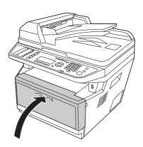
10. Open the MP tray and load the paper back on the MP tray.
