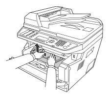
3. Put your finger into the hole of the outer green knob on each side of the photoconductor unit. Then, pull the photoconductor unit towards you.
