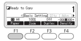
6. Select the paper source using the  $\triangle$  or  $\nabla$  button and press the **OK** button.
