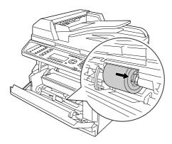
2. Slide the locking lever to the right until it stops, and insert the gray rod into the hole on the pickup roller.
