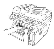
5. Put your finger into the hole of the outer green knob on each side of the photoconductor unit. Then, pull the photoconductor unit towards you.
