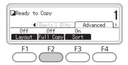
3. Select On using the ▲ or ▼ button and press the **OK** button.
