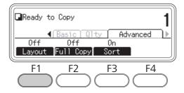
5. Select On using the ▲ or ▼ button and press the **OK** button.
