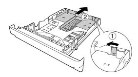
3. Load a stack of the desired paper on the center of the paper cassette with the printable surface facing down.
