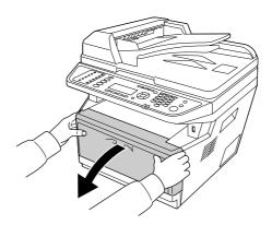
4. Remove the developer unit containing the toner cartridge.
