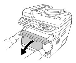
2. Remove the developer unit containing the toner cartridge.
