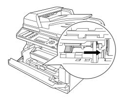
3. Push the locking lever up to lock the pickup roller.
