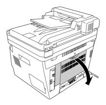
2. Pull the green labeled lever down and gently pull any sheets of paper out.
