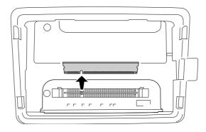
6. Insert the memory module into the memory slot until it stops.
