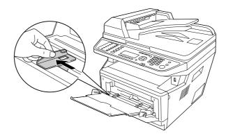
3. Load a stack of the desired paper on the center of the paper tray with the printable surface facing up. Then adjust the paper guide to the size of the paper.
