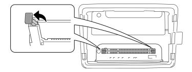
5. Remove the memory module from the memory slot.
