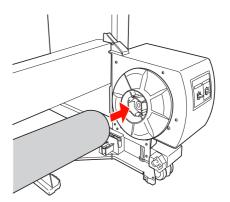
Insert the flanged knob on the movable unit into the other end of the take-up reel core.
