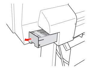
Put the used maintenance tank in the plastic bag provided with the replacement cartridge, and dispose of it properly.
