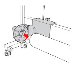
Turn the lock lever to the front to lock the movable unit.
