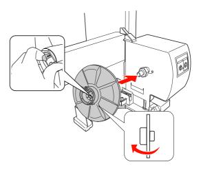
Remove the flange by pinching the knob.
