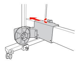
Slip one end of the take-up reel core over the flanged knob on the drive unit.
