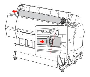
Slide the adapter holder with the handle to make the left roll media adapter align with • on the adapter holder.
