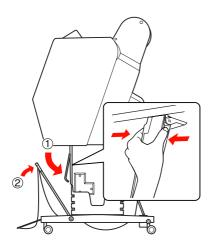
Bring the front paper basket up and fasten it with the hook-and-loop fastener straps.
