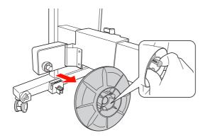
Reverse the flange so that the smaller knob is positioned on the outside, then replace it on the movable unit by pinching the knob.
