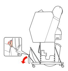
3 Slightly tilt the front paper basket to set the paper guides to the horizontal position.
