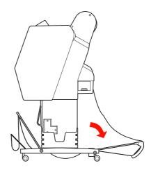
Tilt the front basket until parallel to the floor when ejecting your prints.
