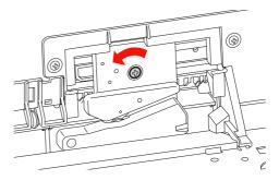
9 Carefully remove the old cutter from the printer.
