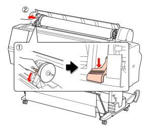
Roll over the paper roll to the front side, and then place it in the gap on the top face of the printer.
