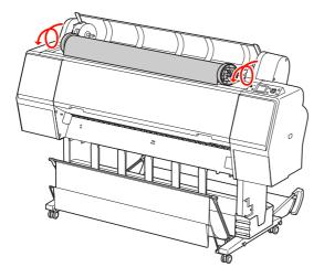
Pull up the lock lever of the adapter to unlock. Then remove the roll media adapter from the paper roll.
