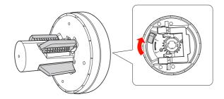
Release the lock lever of the adapters on both sides.
