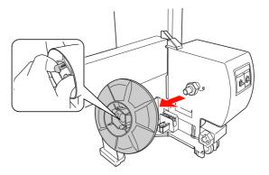
Reverse the flange so that the smaller knob is positioned on the outside, then replace it on the drive unit by pinching the knob.
