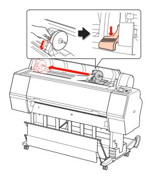
Place the paper roll in the gap on the top face of the printer.
