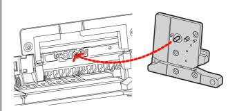
Screw up the cutter firmly with a cross head screwdriver.
