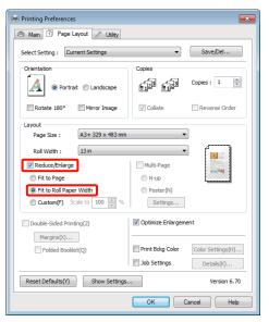
Select the width of the roll paper loaded in the 4 printer from the Roll Width list.
