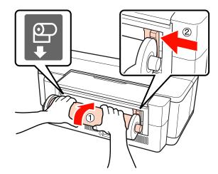
Slide the roll paper in until it stops and keep it lightly held in this position for about three seconds.
