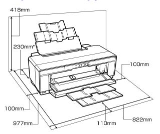
\* When printing on thick paper, leave a space of at least 320 mm behind the printer.
