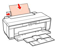
Slide the paper in until it stops and keep it lightly held in this position for about three seconds.
