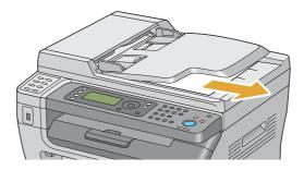
4. Remove any paper in the center output tray if there is. Close the output tray extension if it is extended.
