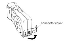
5. Depending on the type of cable you have, line up either the arrow or the flat surface of the long cable connector with the mark on the camera's serial port. Then insert the connector.
