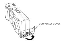
5. Depending on the type of cable you have, line up either the arrow or the flat surface of the cable connector with the mark on the camera's serial port. Then insert the connector.
