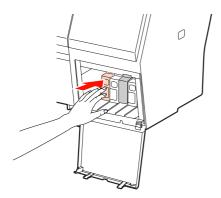
6 Carefully pull the expended cartridge straight out of the slot.
