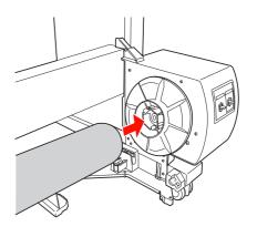
Insert the flanged knob on the movable unit into the other end of the take-up reel core.
