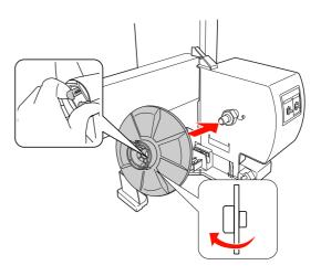
Remove the flange by pinching the knob.
