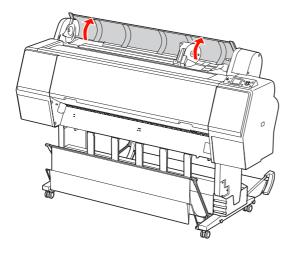
To unlock the adapter holder, push the lock lever of the adapter holder down firmly. Then move the adapter holder to the left with the handle.
