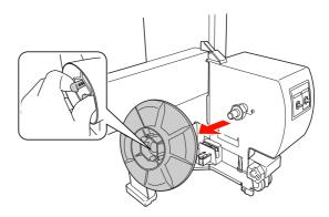
Reverse the flange so that the smaller knob is positioned on the outside, then replace it on the drive unit by pinching the knob.
