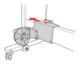
Slip one end of the take-up reel core over the flanged knob on the drive unit.
