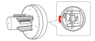
Release the lock lever of the adapters on both sides.
