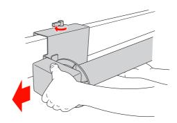
Remove the take-up reel core from the flange knob on the movable unit and the drive unit.
