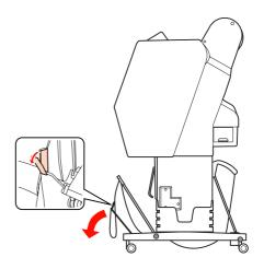
3 Slightly tilt the front paper basket to set the paper guides to the horizontal position.
