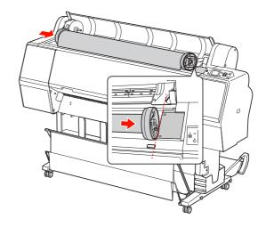
Slide the adapter holder with the handle to make the left roll media adapter align with  $\triangle$  on the adapter holder.
