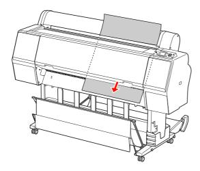
Make sure that the right and bottom edges of the sheet are straight and in line with the set line.
