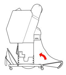
Remove the hook-and-loop fastener straps of the front paper basket, and tilt it down.
