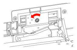
Garefully remove the old cutter from the printer.
