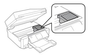
Secure the ink cartridge holder to the case with tape as shown, then close the scanner unit slowly.
