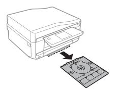
Place a CD/DVD on the CD/DVD tray with the printable side face-up, and then insert the tray into the product. Make sure that the ▲ marks on the tray and the ▼ marks on the product match, so that the line on the tray aligns with the product.
