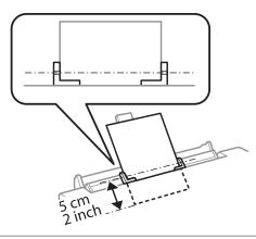
Load the envelope short edge first with the flap facing down and at the center of the rear paper feed slot, and then set the edge guide.
