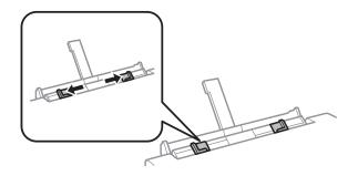
4 Load a single sheet of paper with the printable side face-up at the center of the rear paper feed slot, and then set the edge guide. The printable side is often whiter or brighter than the other side.
