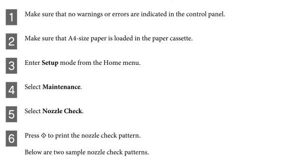
Compare the quality of the printed check page with the sample shown below. If there are no print quality problems, such as gaps or missing segments in the test lines, the print head is fine.
