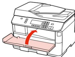
Insert the cartridge into the slot until it clicks and close the cover. Initial ink charging will automatically start. It takes about 7 minutes. Wait until a completion message is displayed on the LCD screen.
