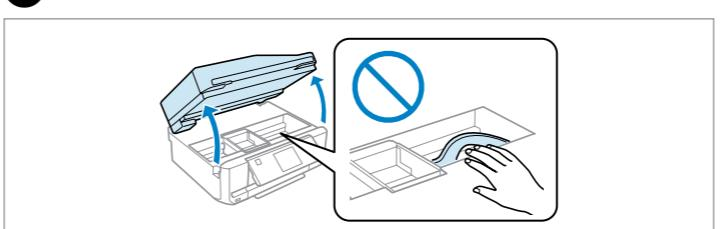
When instructed to install the cartridges, open the upper section.
