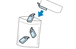
Install the ink cartridges head first.
