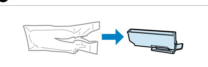
Remove the ink cartridge from its package.
