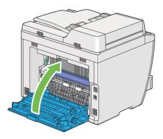
If the error is not resolved, there may be a piece of paper remaining inside the printer. Use the following procedure to clear the jam.
