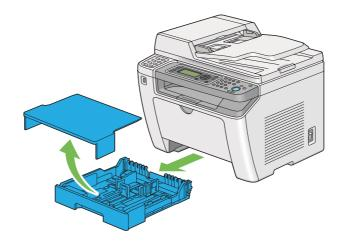
2. Hold the paper tray end with one hand, push and hold the paper tray extension lever with the other hand, and then extend the tray to your desired length.
