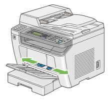
3. Before loading the print media, flex the sheets back and forth, and then fan them. Straighten the edges of the stack on a level surface.
