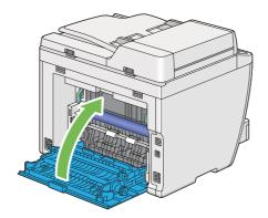
If the error is not resolved, there may be a piece of paper remaining inside the printer. Use the following procedure to clear the jam.
