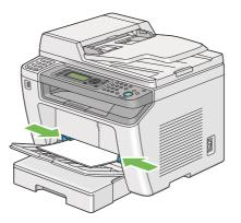
6. Select the paper type on the print driver if the loaded print media is not plain paper. If a user-specified print media is loaded in the PSI, you must specify the paper size on the print driver.
