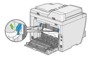
3. Remove the jammed paper from the rear of the printer.
