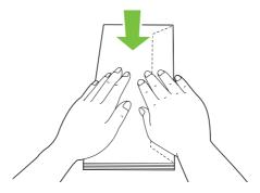
□ If envelopes are still not fed correctly, add some bending to the flap of the envelopes as shown in the following illustration. The amount of the bending shall be 5 mm (0.20 inches) or less.
