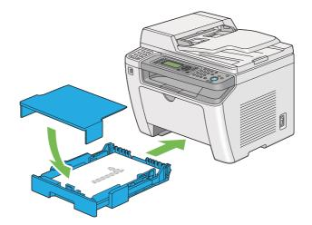
2. After the even pages are printed, pull out the paper tray and remove the paper tray cover.
