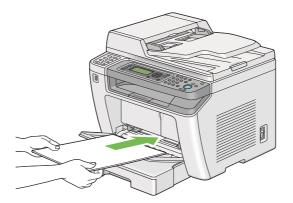
5. Slide the paper width guides inward until they rest lightly against the edges of the print media stack.
