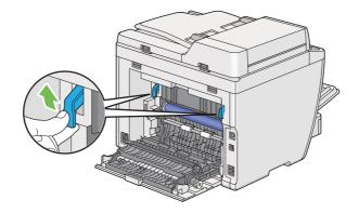
3. Pull the jammed paper out carefully to avoid tearing it.
