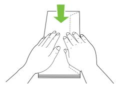
□ If envelopes are still not fed correctly, add some bending to the flap of the envelopes as shown in the following illustration. The amount of the bending shall be 5 mm (0.20 inches) or less.
