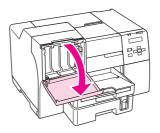
2. Move the cartridge lever to the unlocked position.
