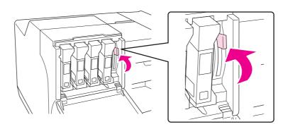
3. Remove the expended installed ink cartridge.
