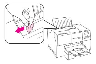
4. Load envelopes short edge first with the flap facing down and to the left. Then slide the left edge guide against the left edge of the envelopes.
