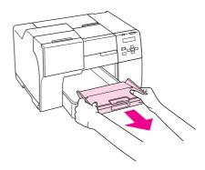
2. Slide the output support tray until it clicks. The output support tray is lifted slightly.
