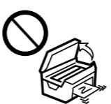
Do not open the scanner unit while copying, printing, or scanning.
