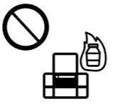
Do not use aerosol products that contain flammable gases inside or around the printer. Doing so may cause fire.
