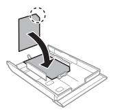
Use cassette 2 when loading envelopes. Load envelopes short edge first with the flap facing up and to the left. Next, check that the envelopes are not sticking out from the end of the cassette.
