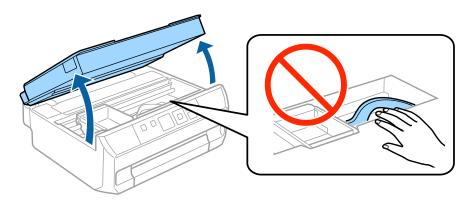
Do not touch the white flat cable inside the printer.
