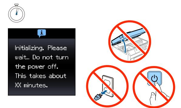
The initial ink cartridges will be partly used to charge the print head. These cartridges may print fewer pages compared to subsequent ink cartridges.
