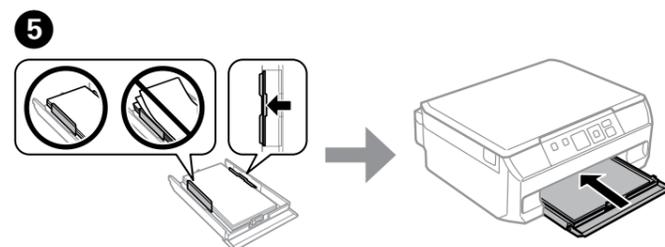
Slide the edge guides to the edges of the paper. Keep the cassette flat and insert it back into the product carefully and slowly.
