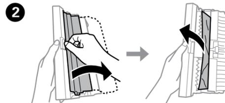
2 Open the rear cover and carefully remove the jammed paper.
