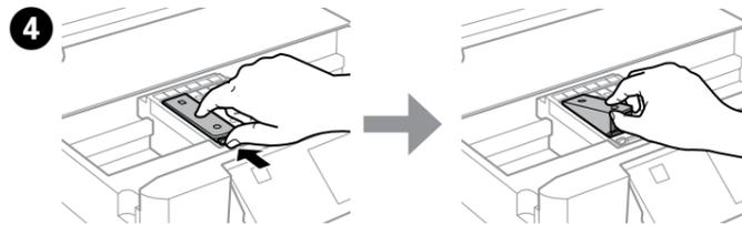
4 Push the tab to unlock the ink cartridge holder and then remove the cartridge diagonally.
