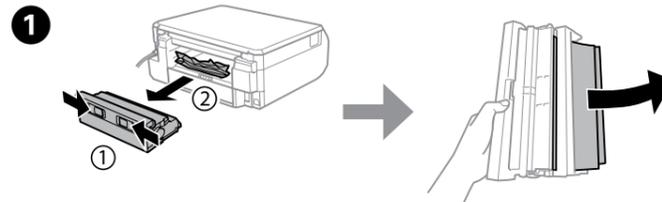
1 Pull out the rear cover and carefully remove the jammed paper.
