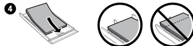
Load paper toward the edge guide with printable side face-down, and check that the paper is not sticking out from the end of the cassette.
