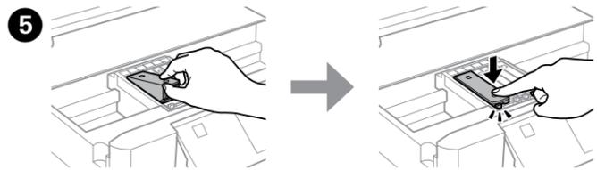
5 Insert the ink cartridge diagonally into the cartridge holder and gently push it down until it clicks into place.
