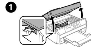
1 Open the scanner unit and remove all of the paper inside, including any torn pieces.
