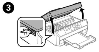
3 Open the scanner unit. The ink cartridge holder moves.
