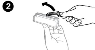
2 Remove the cap from the new cartridge.
