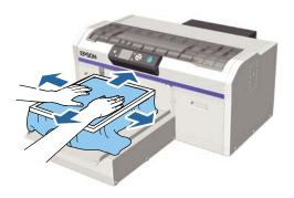
Pull the T-shirt outside of the frame to remove any creases and slack.
