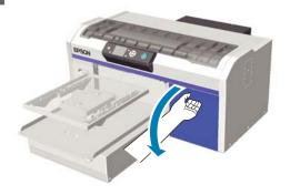
Put your finger into the indentation on top of the ink cartridge and pull it straight out.
