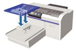
After replacing the platen with a different size, we recommend you correct print misalignment (head alignment).
