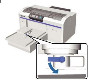
Remove the screw that secures the parallel adjustment plate.
