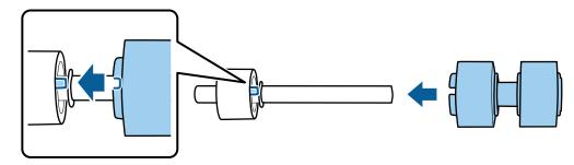
Check that there are no gaps. Make sure the roller does not come off the axis.
