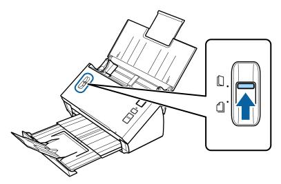
4 Load the card into the input tray with the printed side facing down and the top edge facing into the feeder. Slide the card into the feeder until it meets resistance. Then slide the edge guides to fit the edge of the card.
