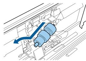
Remove the roller from the axis.
