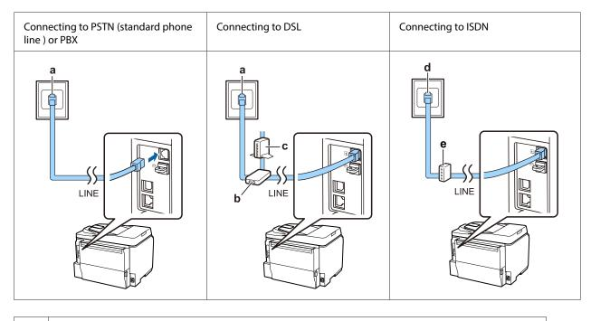
a Telephone wall jack or PBX portIf you have a PBX console in the room, connect the telephone cable from the console to the LINE port.
