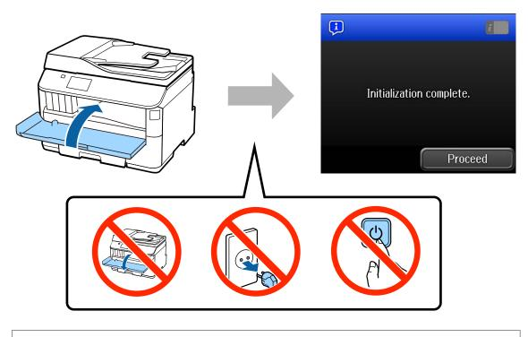
The initial ink cartridges will be partly used to charge the print head. These cartridges may print fewer pages compared to subsequent ink cartridges.
