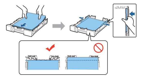
Keep the cassette flat and slowly and carefully reinsert it all the way into the product. Slide out the output tray and raise the stopper.
