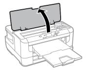
Make sure the ink cartridge holder is at the ink cartridge replacement position.
