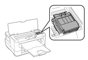
Secure the ink cartridge holder to the case with tape as shown.
