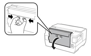
Put your hand on the handle of the maintenance box, and then pull the box outward.
