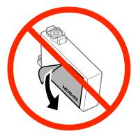
Do not remove the transparent seal from the bottom of the cartridge; otherwise, the cartridge may become unusable.
