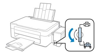
Unhook the ink tank unit from the product and lay it down, and then make sure to install the cap onto the ink tank securely.
