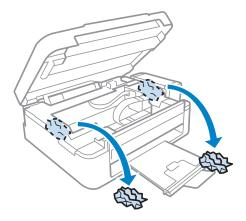
Close the scanner unit. If the jammed paper remains near the output tray, carefully remove the paper.
