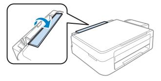
Slide out the paper support and the output tray and then raise the stopper.
