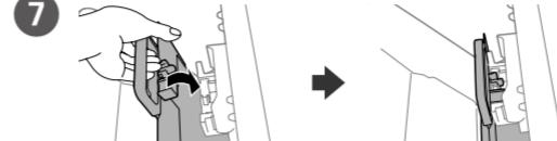
Fit the ink supply port and the green chip into the printer, then push the handle of the ink supply unit.
