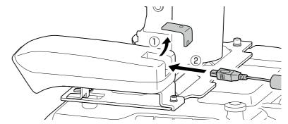
Attach the USB cover, and then secure it using the M3 x 8 mm cross-head screw.
