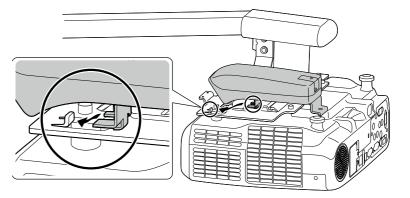
2 Use the M4 x 10 mm bolt with washer and spring washer to secure the Interactive Unit.
