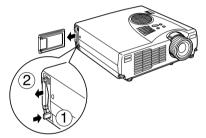
**3** Press the button on the left-hand side of the PCMCIA card slot if it is protruding. This will restore the button in its original place.
