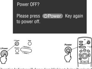
The Operation Indicator will change from blinking to being illuminated in orange once the cool-down process has been completed. The cool-down period will take approximately ninety seconds (depending on the surrounding temperature).
