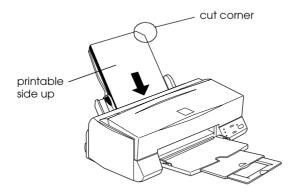
☐ Make sure the paper stack fits under the arrow mark located on the inside surface of the left edge guide.
