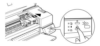
The printer starts cleaning the print head and the  $^{\circlearrowleft}$  power light begins flashing. Print head cleaning takes about one minute to complete.
