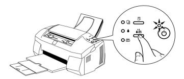
The EPSON Stylus Scan starts cleaning the print head and the  $\bigcirc$  power light begins flashing. Print head cleaning takes about one minute to complete.
