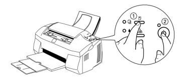
The Stylus Scan prints an operation check page including its ROM version information, the ink counter code, and a nozzle check pattern. Below are sample printouts.
