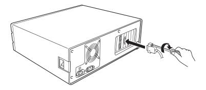
3. Plug the 36-pin end of the cable into the scanner's interface connector. Then squeeze the wire clips together until they lock in place on both sides.
