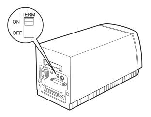
If the scanner is the only SCSI device you connect to your computer or if it is the last device in the daisy chain, leave the internal SCSI terminator turned on.
