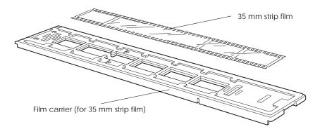
1. Place the film carrier on a table or other stable surface, and take off the upper half. Hold the sides with one hand, and use the other hand to completely remove the upper half, as shown below.
