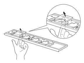
2. Grasp the edge of the slide and pull it out gently in the direction shown below.
