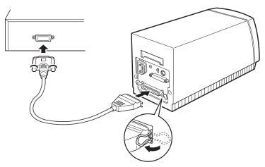
An example using the scanner's 50-pin interface.
