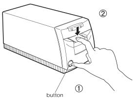
6. Insert the cartridge holder into the scanner with the arrow marks first as shown below.
