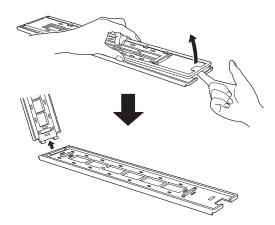
2. Load the film into the carrier between the small tabs, with the film's base side facing up. The film maker's name and film ID numbers are shown on the base side.
