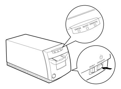
5. Make sure the READY light is on, then push the film carrier about half-way into the scanner as shown below. The scanner slides the carrier backward and forward, and when the READY light comes on again, the film is in the correct position.
