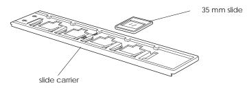
1. Hold the slide carrier so that the arrows face up, then insert your slide, face up, under one of the sets of tabs as shown below. When you look at the slide from this side of the carrier, the image in the slide should appear in its correct orientation.
