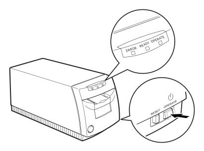
3. Make sure the READY light is on, then load the film carrier about half-way into the scanner with the arrow marks first as shown below. The scanner slides the carrier backward and forward, and the film carrier is in the correct position when the READY light comes on again.
