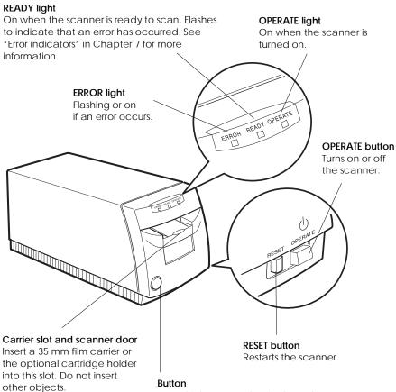
Press this button and push down the scanner door before inserting the optional cartridge holder into the scanner. Be sure to push down the scanner door again to close the door.
