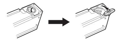
2. Insert the film cartridge into the holder in the manner shown below. Then close the cover and turn the knob to the LOCK position.
