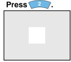
A spotlight appears on the screen. The size of the spotlight changes to one of three sizes each time the button is pressed.
