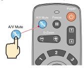
First press the \_\_\_\_\_ button, select "Setting" and then "A/V Mute". Then select the type of screen to be displayed when projection is being stopped. The following choices are available. The default setting is the black screen.
